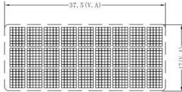
Figure 8: Schematic of the Dot Matrix LC Display (unit: mm)
