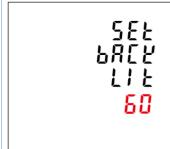
The meter provides a function to set the backlit lasting time.
