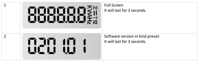
After the self-checking program, the meter display will show the total active energy (kWh)
