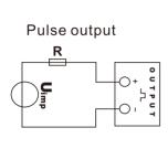
ATTENTION: Pulse output must be fed as shown in the wiring diagram above. Scrupulously respect polarities and the connection mode. Opto-coupler with potential -free SPST-NO Contact. Contact range: 5~27V DC Max. Current Input: 27mA DC.
